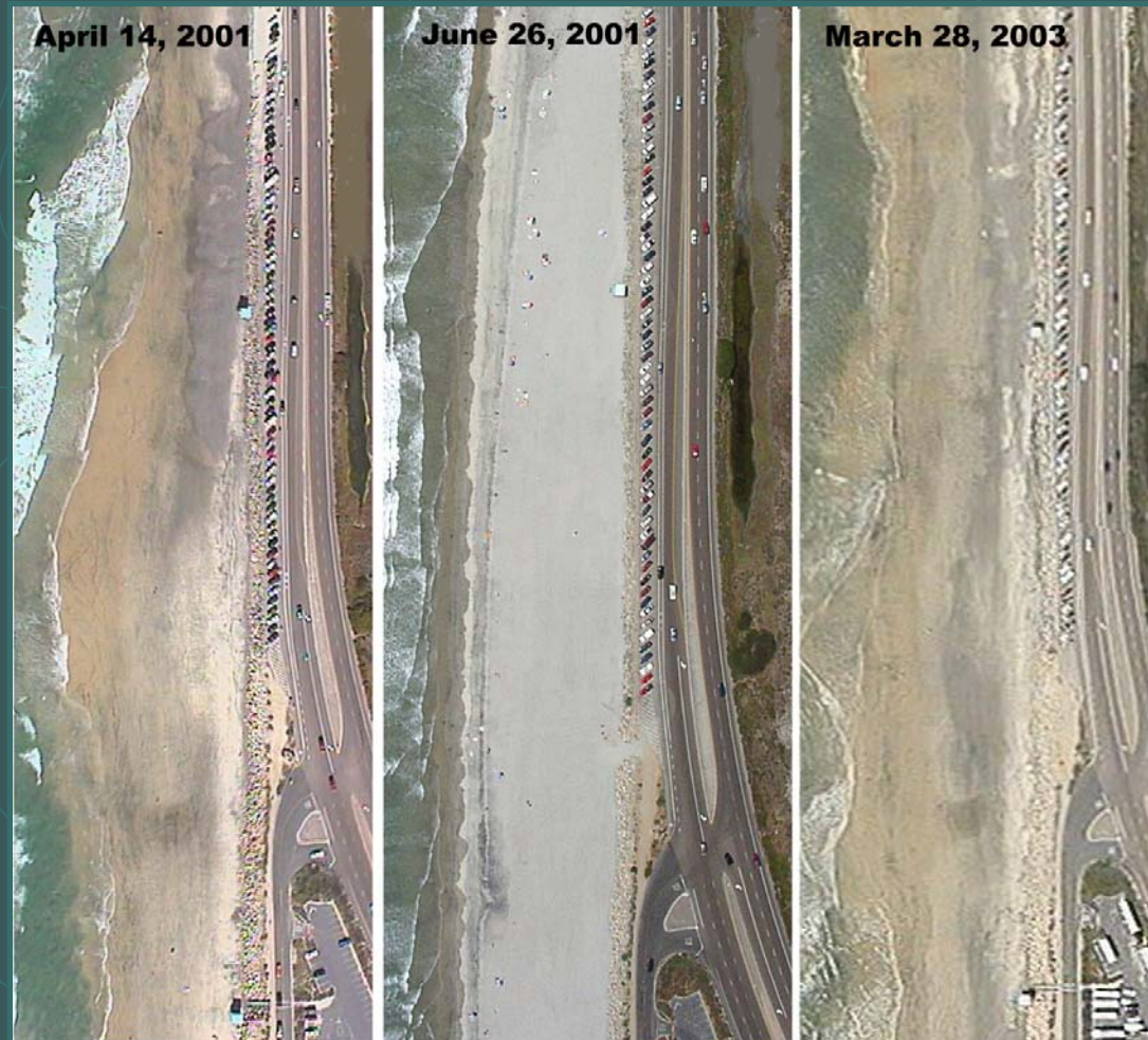
Photograph showing Torrey Pines Beach before and after 260,000 yd 3 of sand placement on the beach in April 2001.
