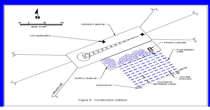
• The front loader is used to place calculated amounts of substrate (rock or concrete).
